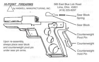
NOTE: When installing sear pin, ramp on top of sear pin faces to the front of handgun.
