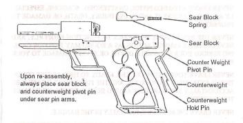
NOTE: When installing sear pin, ramp on top of sear pin faces to the front of handgun.
